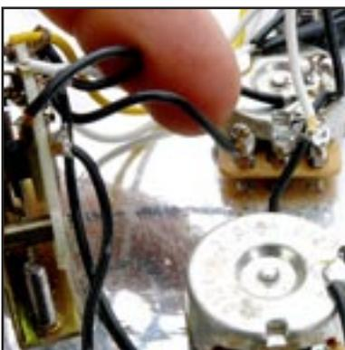
The wire on the left tab of your volume control is the output from the 5-way switch. The middle wire is the output from the volume control- Stock #1 and Mod wiring uses this center wire straight to the Input tab on the MODboard.
