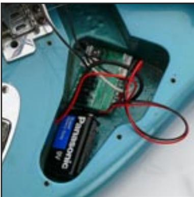
If using Stock Strat Setup #1 you may place the 9 Volt battery under the Tone knob as shown.
