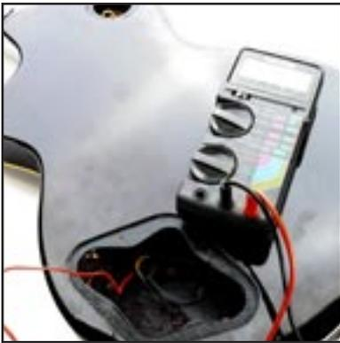
After you connect the pickups to the toggle switch, TEST everything before you go any further. Once you know that both the wire coming back from the toggle switch is getting the output of both pickups, you're OK.
