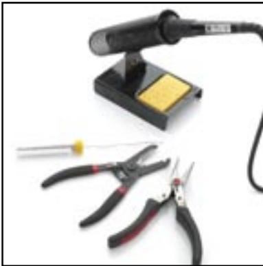
Correct installation requires the correct tools. We recommend a high quality 30-40 watt soldering station, high quality wire strippers, pliers and cutters, and only use correct 60/40 solder when working on MODboards
