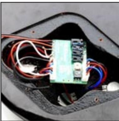
Once the volume and tones are installed it's time to wire up the MODboard. You can install the output jack first, then the battery leads, then the input from the volume pot. Remember to connect INPUT ground to the back of the volume pot.
