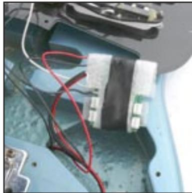
Using the supplied cellular foam, make a wrap for the board. If space is tight you can use thin cardboard to create a shield for the board, or lightly wrap it in electrical tape. It is very important that the bottom of the MODboard is covered to prevent shorting.
