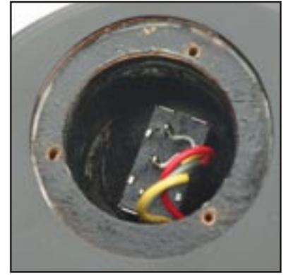
We need to look at our toggle switch and check to see which side is neck and which side is bridge. Most guitars are color coded, but even if you're wrong you can rotate the switch 180 degrees to be correct.
