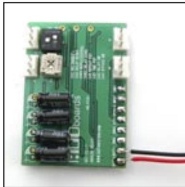
If you *can* mount the battery in the cavity, you'll want to install the battery leads now- Trim the leads so you don't have too much extra wire, and solder the black and red as shown.
