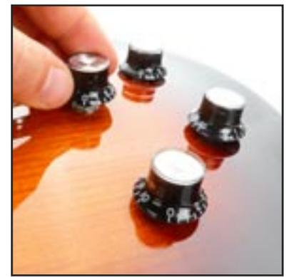
Once installed everything looks stock! By pulling up on the volume pot we can engage the MODboard, and this control STILL operates as the standard passive volume control.
