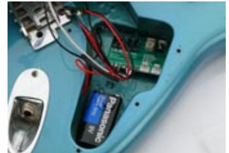
You'll want to measure your cavity thoroughly including depth, and then decide on controls that will fit depth-wise, as well as a good battery location. (A 9 volt battery is 26mm x 17mm x 48mm)
